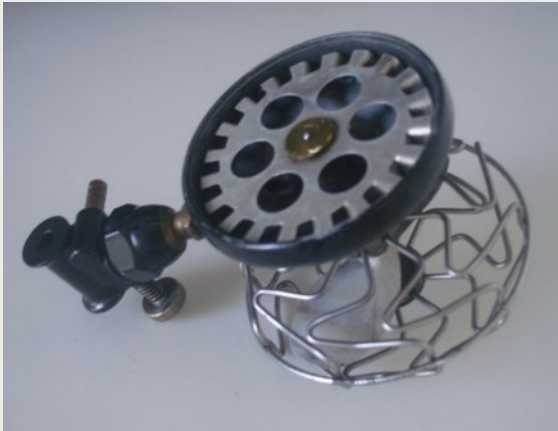
Trico vacuum fan with back cover removed
