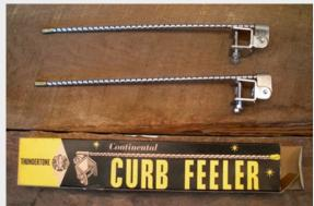
accessory. They clearly alerted the driver to curb on the passenger side of the car. Curb feelers helped to protect 50s American cars from "curb rash" damage to their whitewall tires, large hubcaps, rear wheel skirts and the portly low-hung bodies of the period. There were several companies that offered their own version of curb feelers, but they were all basically the same.
