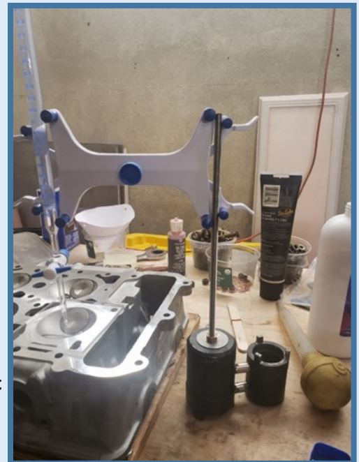
Checking the combustion chamber volumes:
