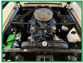
tion. I adjusted the valves, replaced the valve cover gaskets, the oil pan gasket, the transmission pan filter and gasket, and the fuel pump. The headlights and marker lights have been updated to LEDs. New Magnum 500 wheels and raised white letter tires updated the look and stance. Next up is a rebuild of the heater
